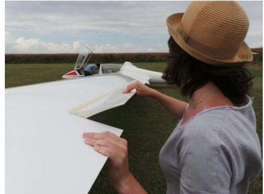
**Pre-flight inspection - Flight control check
